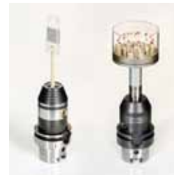
Calibrated ruby sphere gauges mounted on a high precision part holder to validate the compliance of specified MPE_{SD}
